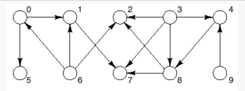
Then, a <u>topological ordering</u> of the vertices in G is a sequential listing of the vertices such that for any pair of vertices, v and w in G, if (v,w) is an edge in G then v precedes w in the sequential listing.
