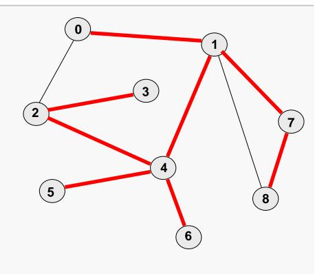
If we modify DFS() to take another AdjMatrix object as a parameter, it is relatively trivial to have DFS() build a copy of the spanning tree.
