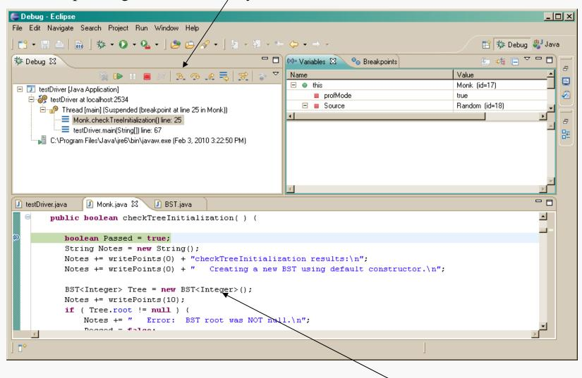
Click the Step-into button until the highlight reaches the instantiation of a BST object...
