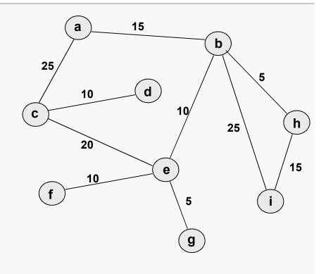
By modifying Dijkstra's SSAD Algorithm to build a list of the edges that are used as vertices are added, and storing the distance from nodes to the current tree (rather than from nodes to the source) we obtain Prim's Algorithm (V Jarnik, 1930 and R C Prim, 1957).
