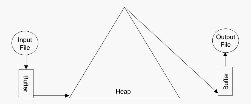
Fill the heap, heapify, and delete the root to the output buffer. If the next key in the input buffer is larger than the old root, make it the new root, else...
