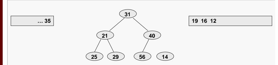
... and so forth ... when the heap becomes empty, we just flush the buffer out to the file, heapify the array (which is where?) and begin a new run...
