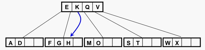
The immediate predecessor is copied to replace the value being deleted and then removed from the leaf (trivial case this time):
