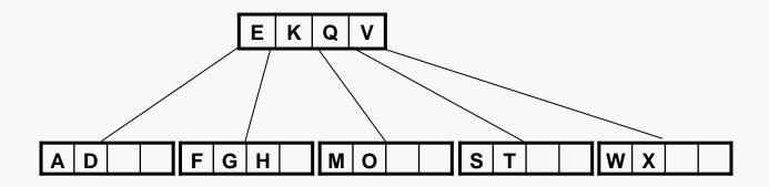
Removing **T** from the leaf causes it to "underflow".
