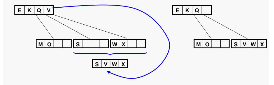
Deleting a value from an internal node is accomplished by reducing it to the former case.
