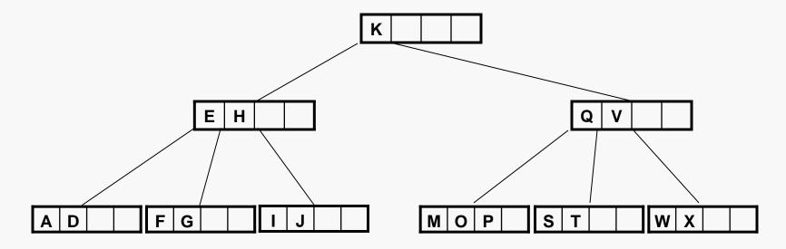
So, the B-tree grows by pushing up a new root, which keeps all leaves at the same level.
