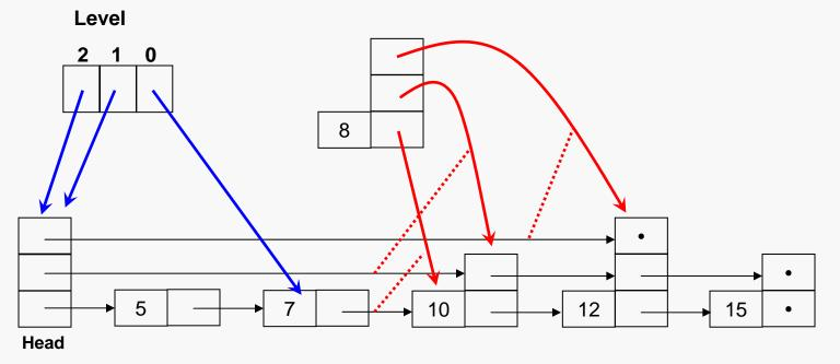
The pointers <u>from</u> the new node are set using the pointers identified earlier, taking into account the levels.
