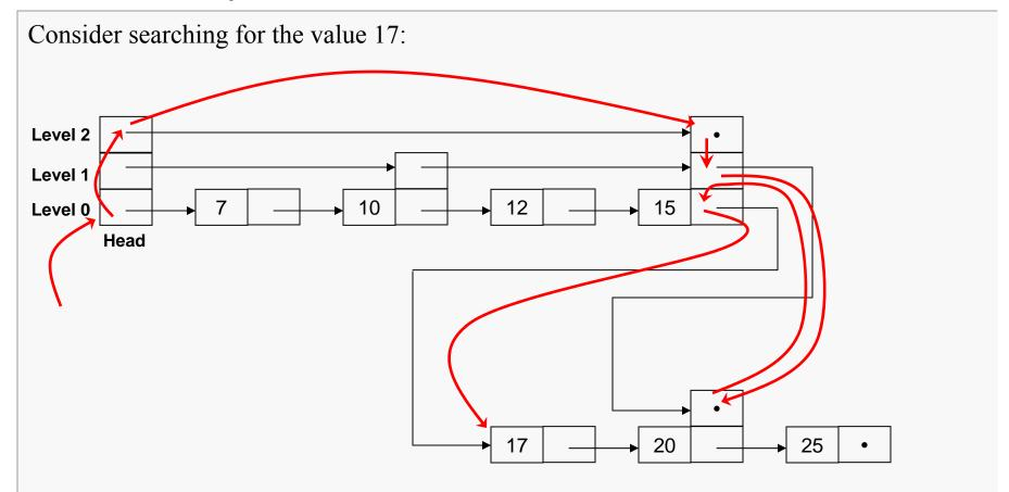
By using the extra pointers, we can jump over the first half of the list, and then determine that the value does not lie within the fourth quarter of the list. A careful count of operations doesn't show any advantage for this tiny list, but...
