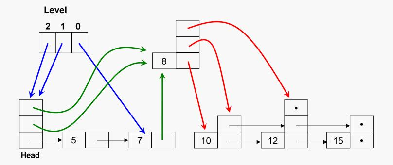
In practice, resetting the pointers <u>from</u> and <u>to</u> the new node would be interleaved so only one pass through the list of "passed" pointers is needed.
