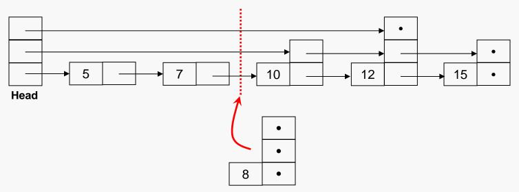
The first step is to search for the largest value already in the list that is less than or equal to the new value. The new node will become the level-0 successor of that existing node.
