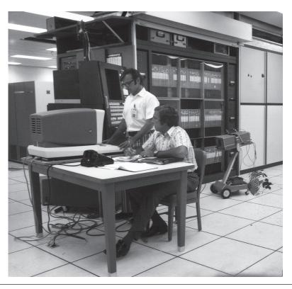
**FIGURE 7.14.1 The Illiac IV control unit followed by its 64 processing elements.** It was perhaps the most infamous of supercomputers. The project started in 1965 and ran its first real application in 1976. The 64 processors used a 13-MHz clock, and their combined main memory size was 1 MB: 64 × 16 KB. The Illiac IV was the first machine to teach us that software for parallel machines dominates hardware issues. Photo courtesy of NASA Ames Research Center.
