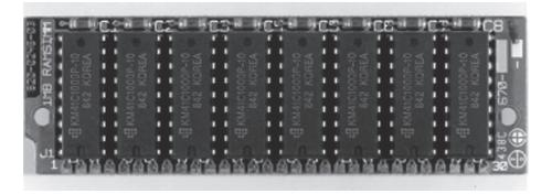
**FIGURE 5.13.4 A 1 MB SIMM, built in 1986, using 1 Mbit chips.** This SIMM sold for about \$5/MB in 1997. As of 2006, most main memory is packed in DIMMs similar to this, though using much higher-density memory chips (1 Gbit).
