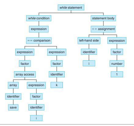
**FIGURE 2.15.2** An abstract syntax tree for the *while* example. The roots of the tree consist of the informational tokens such as numbers and names. Long chains of straight-line descendents are often omitted in constructing the tree.
