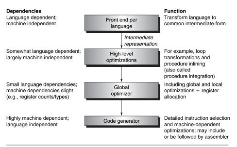
**FIGURE 2.15.1** The structure of a modern optimizing compiler consists of a number of **passes or phases.** Logically, each pass can be thought of as running to completion before the next occurs. In practice, some passes may handle a procedure at a time, essentially interleaving with another pass.
