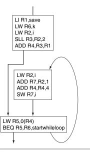
FIGURE 2.15.5 The control flow graph showing the representation of the *while* loop example after code motion and induction variable elimination. The number of instructions in the inner loop has been reduced from 10 to 6.
