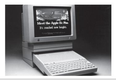
**FIGURE 1.10.5** The Apple IIe Plus. Designed by Steve Wozniak, the Apple IIe set standards of cost and reliability for the industry.
