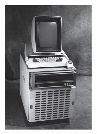
**FIGURE 1.10.6** The Xerox Alto was the primary inspiration for the modern desktop **computer.** It included a mouse, a bit-mapped scheme, a windows-based user interface, and a local network connection.
