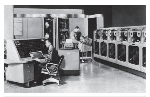
**FIGURE 1.10.2 UNIVAC I, the first commercial computer in the United States.** It correctly predicted the outcome of the 1952 presidential election, but its initial forecast was withheld from broadcast because experts doubted the use of such early results.
