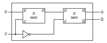
**FIGURE C.8.4 A D flip-flop with a falling-edge trigger.** The first latch, called the master, is open and follows the input *D* when the clock input, *C*, is asserted. When the clock input, *C*, falls, the first latch is closed, but the second latch, called the slave, is open and gets its input from the output of the master latch.
