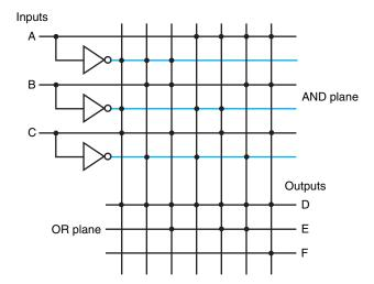
**FIGURE C.3.5** A PLA drawn using dots to indicate the components of the product terms and sum terms in the array. Rather than use inverters on the gates, usually all the inputs are run the width of the AND plane in both true and complement forms. A dot in the AND plane indicates that the input, or its inverse, occurs in the product term. A dot in the OR plane indicates that the corresponding product term appears in the corresponding output.
