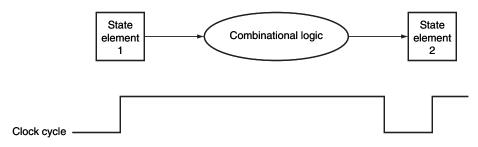
FIGURE C.7.2 The inputs to a combinational logic block come from a state element, and the outputs are written into a state element. The clock edge determines when the contents of the state elements are updated.
