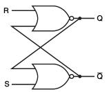
**FIGURE C.8.1** A pair of cross-coupled NOR gates can store an internal value. The value stored on the output Q is recycled by inverting it to obtain  $\overline{Q}$  and then inverting  $\overline{Q}$  to obtain Q. If either R or  $\overline{Q}$  is asserted, Q will be deasserted and vice versa.
