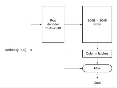
**FIGURE C.9.6** A 4M × 1 DRAM is built with a 2048 × 2048 array. The row access uses 11 bits to select a row, which is then latched in 2048 1-bit latches. A multiplexor chooses the output bit from these 2048 latches. The RAS and CAS signals control whether the address lines are sent to the row decoder or column multiplexor.
