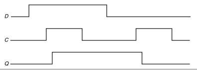
**FIGURE C.8.3** Operation of a D latch, assuming the output is initially deasserted. When the clock, *C*, is asserted, the latch is open and the *Q* output immediately assumes the value of the *D* input.
