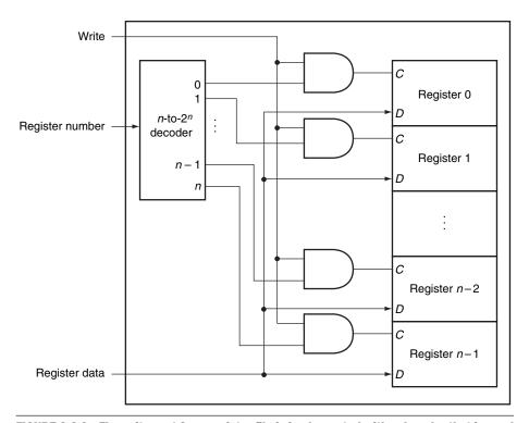
**FIGURE C.8.9** The write port for a register file is implemented with a decoder that is used with the write signal to generate the *C* input to the registers. All three inputs (the register number, the data, and the write signal) will have setup and hold-time constraints that ensure that the correct data is written into the register file.
