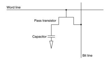
FIGURE C.9.5 A single-transistor DRAM cell contains a capacitor that stores the cell contents and a transistor used to access the cell.
