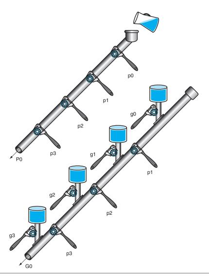
**FIGURE C.6.2** A plumbing analogy for the next-level carry-lookahead signals P0 and G0. P0 is open only if all four propagates (pi) are open, while water flows in G0 only if at least one generate (gi) is open and all the propagates downstream from that generate are open.
