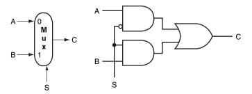
**FIGURE C.3.2** A two-input multiplexor on the left and its implementation with gates on the right. The multiplexor has two data inputs (A and B), which are labeled  $\theta$  and 1, and one selector input (S), as well as an output C. Implementing multiplexors in Verilog requires a little more work, especially when they are wider than two inputs. We show how to do this beginning on page C-23.
