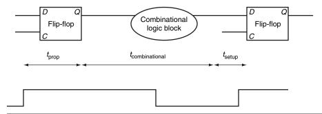
FIGURE C.11.1 In an edge-triggered design, the clock must be long enough to allow signals to be valid for the required setup time before the next clock edge. The time for a flip-flop input to propagate to the flip-flip outputs is  $t_{\text{prop}}$ ; the signal then takes  $t_{\text{combinational}}$  to travel through the combinational logic and must be valid  $t_{\text{setup}}$  before the next clock edge.
