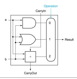
FIGURE C.5.6 A 1-bit ALU that performs AND, OR, and addition (see Figure C.5.5).
