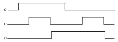
**FIGURE C.8.5** Operation of a D flip-flop with a falling-edge trigger, assuming the output is initially deasserted. When the clock input (*C*) changes from asserted to deasserted, the *Q* output stores the value of the *D* input. Compare this behavior to that of the clocked D latch shown in Figure C.8.3. In a clocked latch, the stored value and the output, *Q*, both change whenever *C* is high, as opposed to only when *C* transitions.
