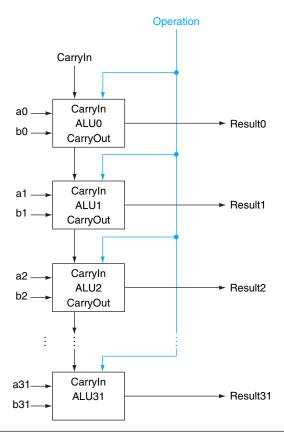
**FIGURE C.5.7** A **32-bit ALU constructed from 32 1-bit ALUs.** CarryOut of the less significant bit is connected to the CarryIn of the more significant bit. This organization is called ripple carry.
