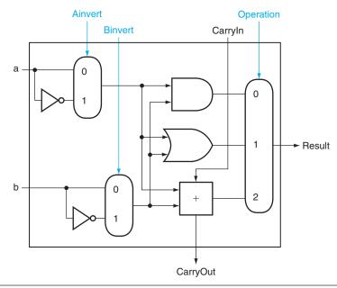
FIGURE C.5.9 A 1-bit ALU that performs AND, OR, and addition on a and b or  $\overline{a}$  and  $\overline{b}$ . By selecting  $\overline{a}$  (Ainvert = 1) and  $\overline{b}$  (Binvert = 1), we get a NOR b instead of a AND b.
