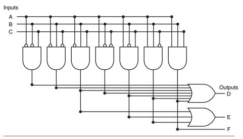
FIGURE C.3.4 The PLA for implementing the logic function described in the example.
