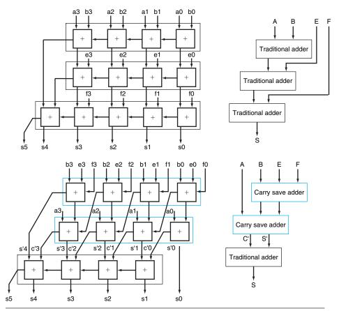
**FIGURE C.14.1 Traditional ripple carry and carry save addition of four 4-bit numbers.** The details are shown on the left, with the individual signals in lowercase, and the corresponding higher-level blocks are on the right, with collective signals in uppercase. Note that the sum of four n-bit numbers can take n + 2 bits.
