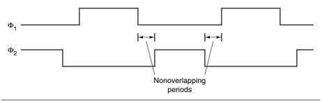
FIGURE C.11.3 A two-phase clocking scheme showing the cycle of each clock and the nonoverlapping periods.
