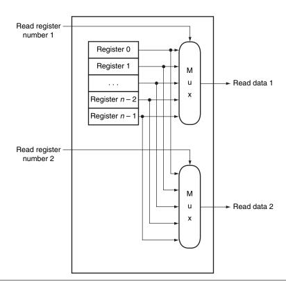
**FIGURE C.8.8** The implementation of two read ports for a register file with *n* registers can be done with a pair of *n*-to-1 multiplexors, each 32 bits wide. The register read number signal is used as the multiplexor selector signal. Figure C.8.9 shows how the write port is implemented.
