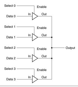
**FIGURE C.9.2** Four three-state buffers are used to form a multiplexor. Only one of the four Select inputs can be asserted. A three-state buffer with a deasserted Output enable has a high-impedance output that allows a three-state buffer whose Output enable is asserted to drive the shared output line.
