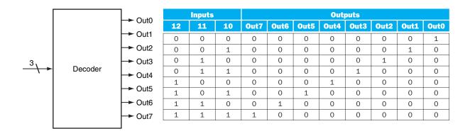
**FIGURE C.3.1** A 3-bit decoder has 3 inputs, called 12, 11, and 10, and 2<sup>3</sup> = 8 outputs, called 0ut0 to 0ut7. Only the output corresponding to the binary value of the input is true, as shown in the truth table. The label 3 on the input to the decoder says that the input signal is 3 bits wide.
