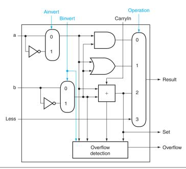
FIGURE C.5.10 (Top) A 1-bit ALU that performs AND, OR, and addition on a and b or  $\overline{\mathbf{b}}$ , and (bottom) a 1-bit ALU for the most significant bit. The top drawing includes a direct input that is connected to perform the set on less than operation (see Figure C.5.11); the bottom has a direct output from the adder for the less than comparison called Set. (See Exercise C.24 at the end of this Appendix to see how to calculate overflow with fewer inputs.)
