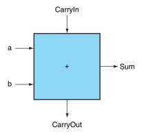
**FIGURE C.5.2 A 1-bit adder.** This adder is called a full adder; it is also called a (3,2) adder because it has 3 inputs and 2 outputs. An adder with only the a and b inputs is called a (2,2) adder or half-adder.
