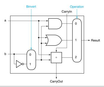
FIGURE C.5.8 A 1-bit ALU that performs AND, OR, and addition on a and b or a and  $\overline{\mathbf{b}}$ . By selecting  $\overline{\mathbf{b}}$  (Binvert = 1) and setting CarryIn to 1 in the least significant bit of the ALU, we get two's complement subtraction of b from a instead of addition of b to a.
