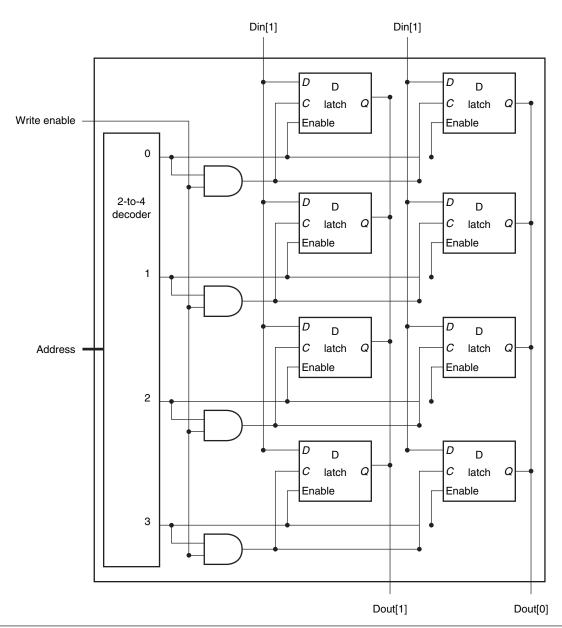
**FIGURE C.9.3** The basic structure of a 4 × 2 SRAM consists of a decoder that selects which pair of cells to activate. The activated cells use a three-state output connected to the vertical bit lines that supply the requested data. The address that selects the cell is sent on one of a set of horizontal address lines, called word lines. For simplicity, the Output enable and Chip select signals have been omitted, but they could easily be added with a few AND gates.
