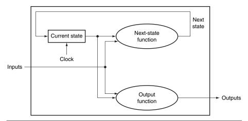
**FIGURE C.10.1** A state machine consists of internal storage that contains the state and two combinational functions: the next-state function and the output function. Often, the output function is restricted to take only the current state as its input; this does not change the capability of a sequential machine, but does affect its internals.
