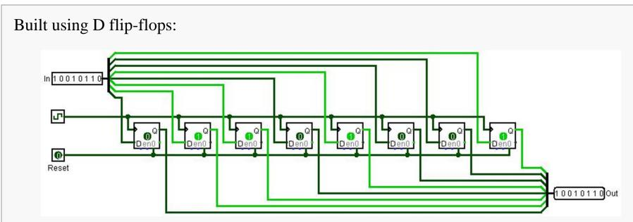
Clock input controls when input is "written" to the individual flip-flops.
