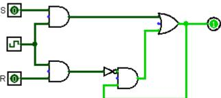
Suppose that the input R is set to 1. Describe precisely how the output value will change as the clock cycles from low to high and back to low.
