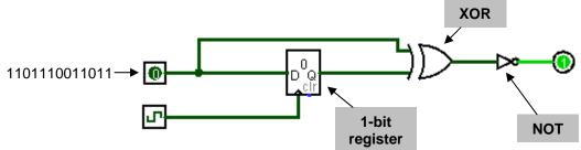
Suppose the input pin on the left side is connected to another circuit that can feed a sequence of bits into it (like a shift register). Assume the clock signal is enabled and that it ticks at exactly the same rate that bits are fed into the input pin.
