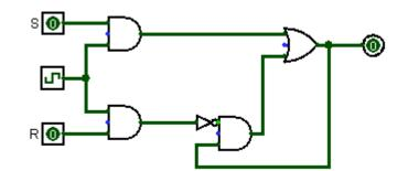
a) [8 points] Suppose that the input S is set to 0 (low). Describe precisely how the output value will change as the clock cycles from low to high and back to low.
