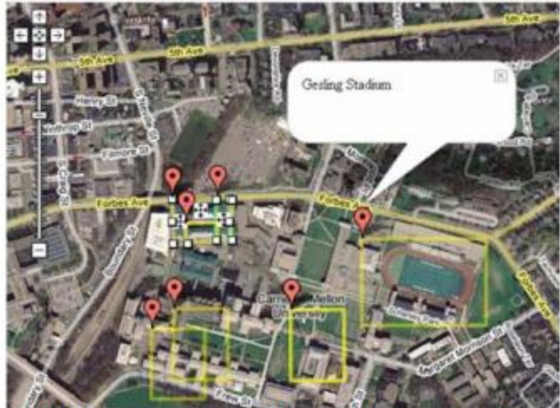
Figure 5. Users can also define locations as combinations of rectangular areas for use in location-sensitive privacy rules.
