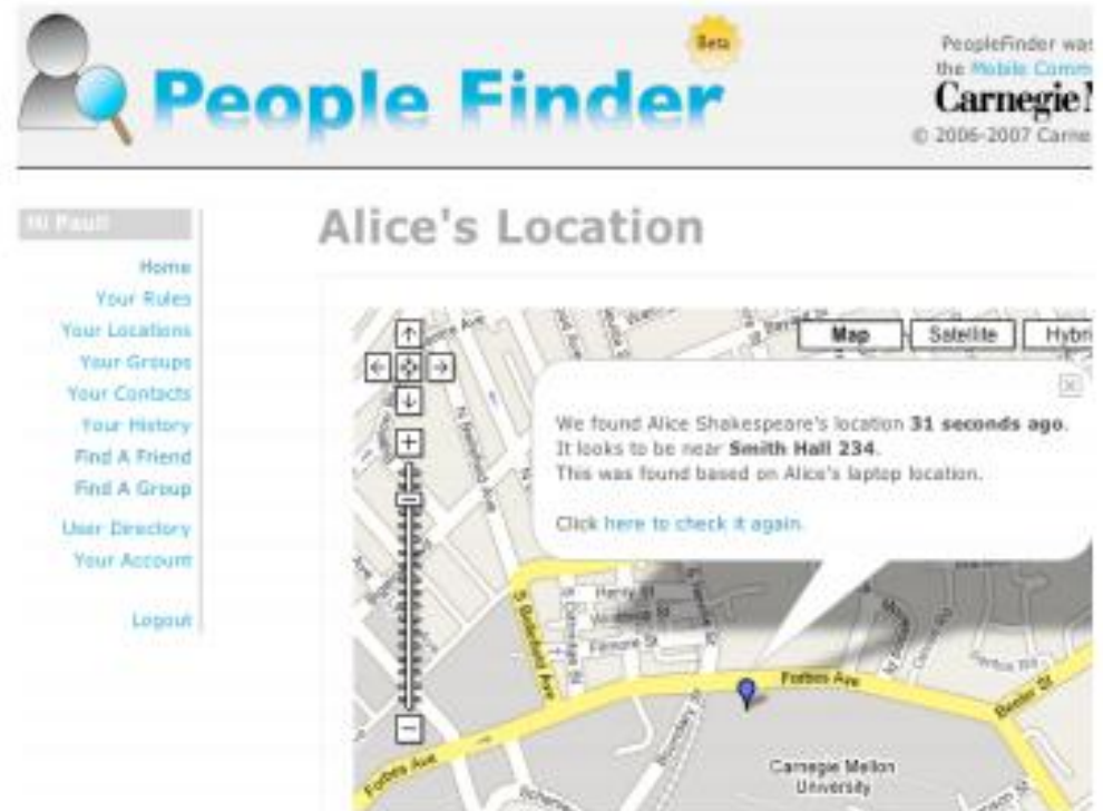
Figure 1. PEOPLEFINDER is an application that lets users share their locations with others subject to privacy policies they can refine over time.
