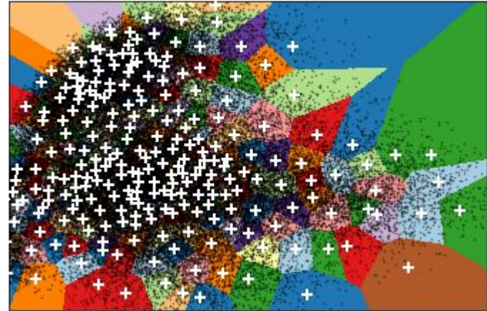
K-means clustering on the digits dataset (PCA-reduced data) 256 Centroids are marked with white dots
