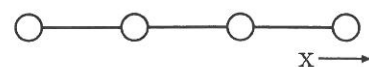
Figure 15.5: A one-dimensional, four-particle HL model. Motion is restricted to the x dimension and is oscillatory.
