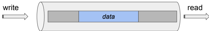
Figure 1: A Unix pipe is a FIFO, bounded buffer that provides the abstraction of a unidirectional stream of bytes flowing from writer to reader
