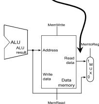
b) [8 points] The MemRead control signal must be set to 0 unless a 1w instruction is being executed. Explain why, for example, a beg instruction could lead to a runtime error if MemRead was set to 1. (Hint: think segfault!)
