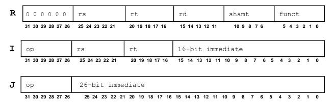
In order to decide how to execute a machine instruction, we would need to know exactly which machine instruction we are dealing with. If the opcode field is 000000, we have an R-format machine instruction, and the funct field tells us exactly which R-format machine instruction we have. Otherwise, the opcode field tells us which machine instruction we have.
