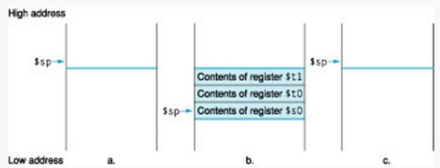
Note that the *run-time stack* is "upside-down". That is, \$sp, decreases when a value is added to the stack and increases when a value is removed.
