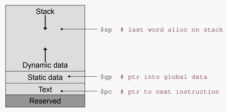
Dynamic data is accessed via pointers held by the program being executed, with addresses returned by the memory allocator in the underlying operating system.
