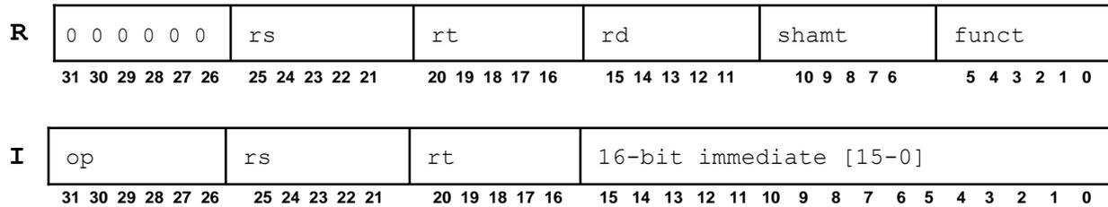
To specify Write register number, R-type instructions use bits 15-11 (rd field), whereas lw instruction (which are I-type) uses bits 20-16 (rt field). This is the reason why the MUX on the left of Registers is needed in the original SCD design. See the SCD diagram included with the test.
