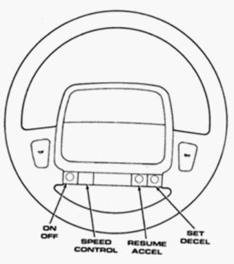
**To Activate** – Push the ON/OFF switch. When depressed the cruise control system is activated. Push the ON/OFF switch again to raise the button and deactivate the cruise control system.
