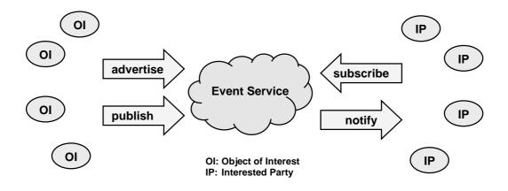
Fig. 7.1. The High-level View of the SIENA Architecture.
