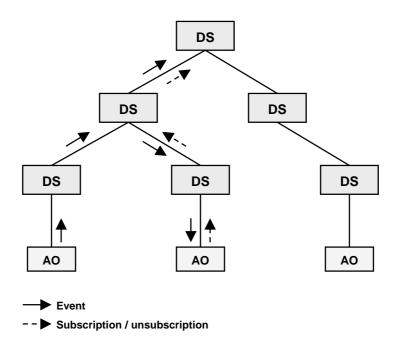
Fig. 6.2. The Structure of Dispatching Servers.
