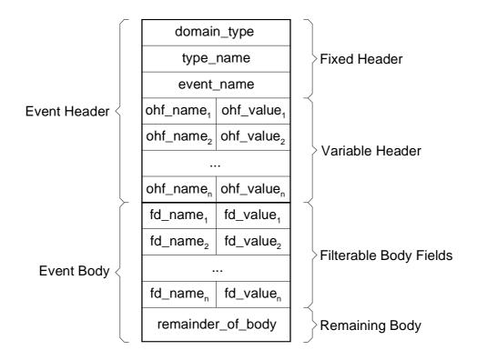
Fig. 2.3. The General Structure of a Structured Event.
