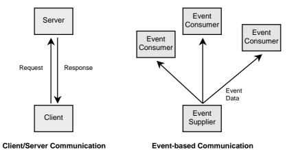
Fig. 1.1. Client/Server and Event-based Computing Models.
