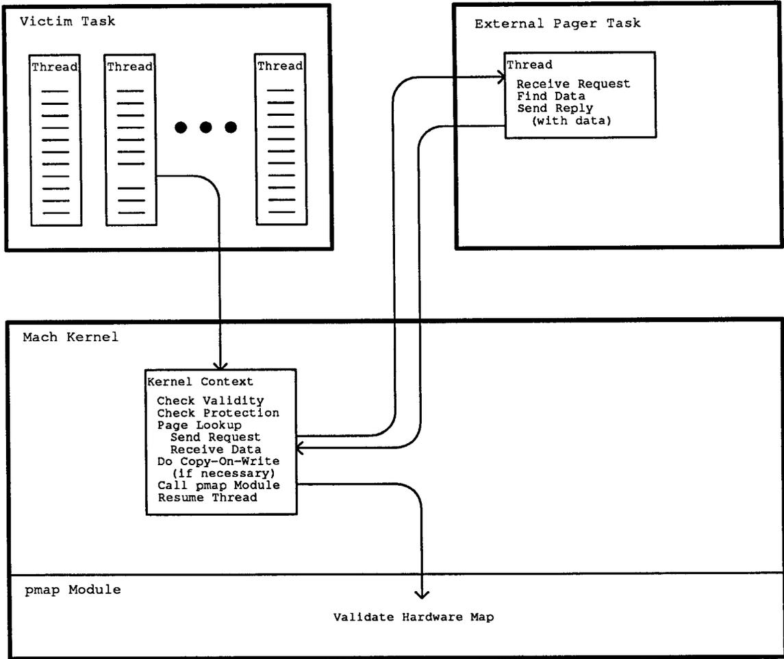
Figure 5-1: Fault Handling
