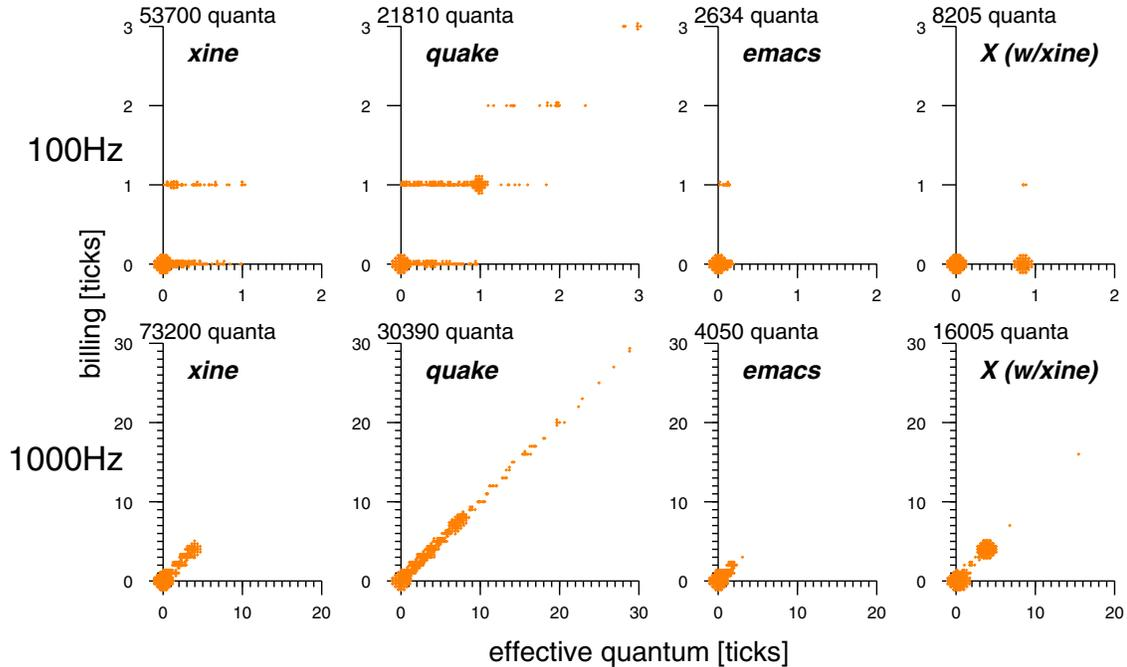
**Figure 4:** The relationship between effective quanta durations and how much the process is billed, for different applications, using a kernel running at 100 Hz and at 1000 Hz. Concentrations of data points are rendered as larger disks; otherwise the graphs would have a clean steps shape, because the billing (Y axis) is in whole ticks. Note also that the optimal would be a diagonal line with slope 1.
