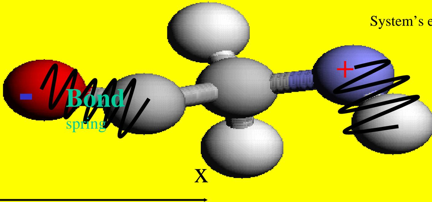
$$E = \underbrace{Kr^2}_{\text{Bond stretching}} + \underbrace{A/r^{12} - B/r^6}_{\text{VDW interaction}} + \underbrace{Q_1Q_2/r}_{\text{Electrostatic forces}} + \dots$$
