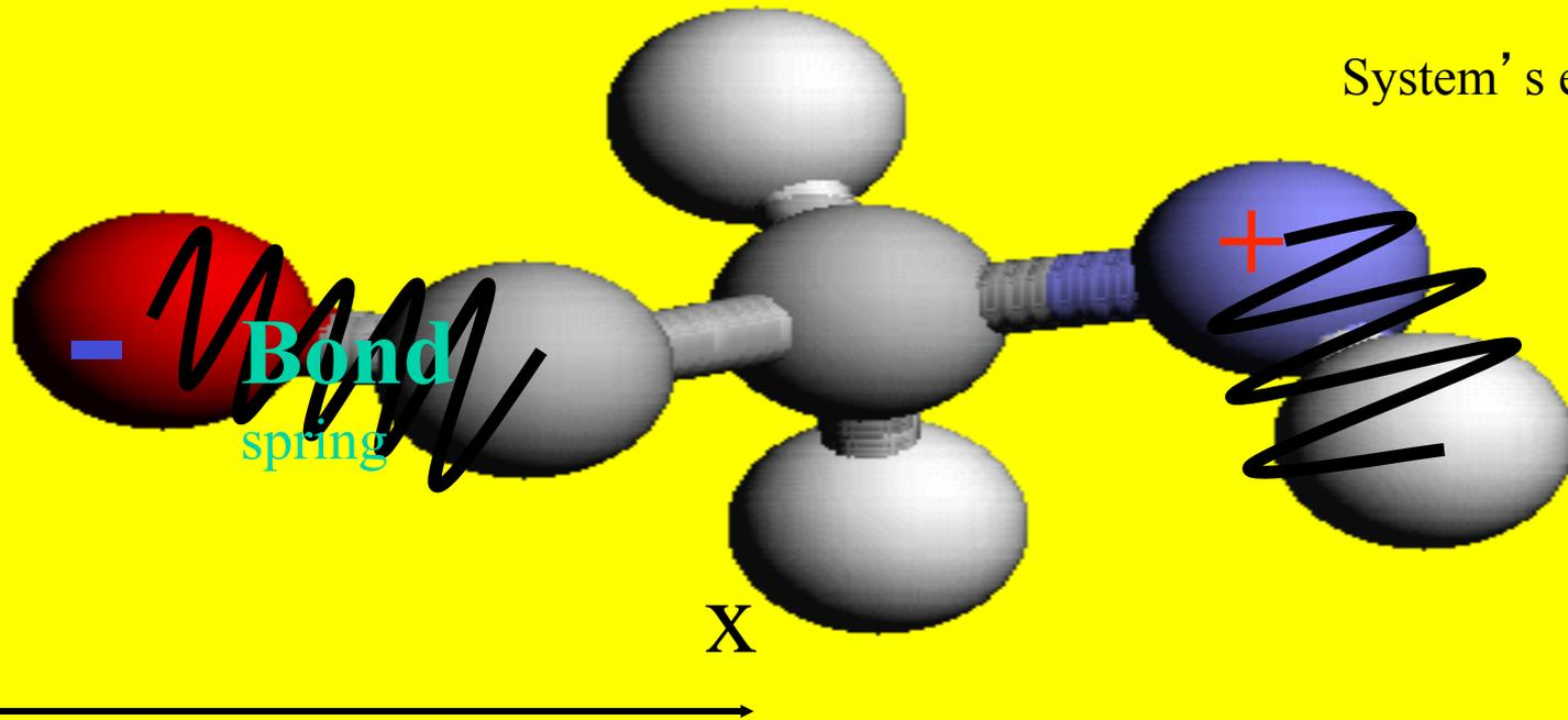
$$E = \underbrace{Kr^2}_{\text{Bond stretching}} + \underbrace{A/r^{12} - B/r^6}_{\text{VDW interaction}} + \underbrace{Q_1Q_2/r}_{\text{Electrostatic forces}} + \dots$$
