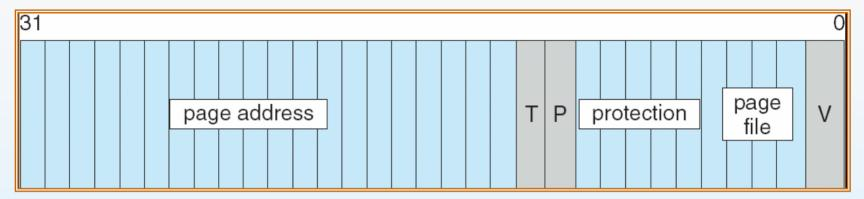
5 bits for page protection, 20 bits for page frame address, 4 bits to select a paging file, and 3 bits that describe the page state. V = 0
