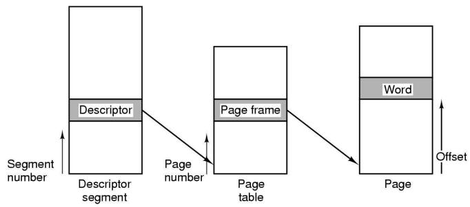
Conversion of a 2-part MULTICS address into a main memory address
