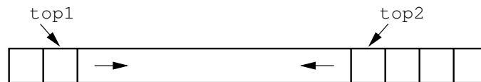
Figure 4.20 Two stacks implemented within in a single array, both growing toward the middle.
