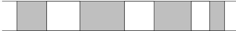
Figure 12.9 Dynamic storage allocation model. Memory is made up of a series of variable-size blocks, some allocated and some free. In this example, shaded areas represent memory currently allocated and unshaded areas represent unused memory available for future allocation.
