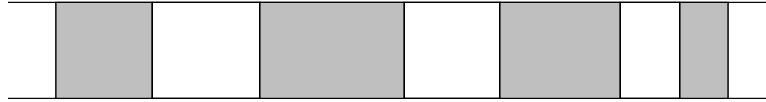
Figure 12.12 Dynamic storage allocation model. Memory is made up of a series of variable-size blocks, some allocated and some free. In this example, shaded areas represent memory currently allocated and unshaded areas represent unused memory available for future allocation.
