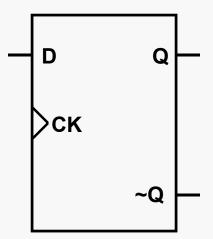
In the following Logisim diagrams, the D flip-flops update state on the falling edge (when the clock goes from high to low).
