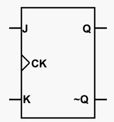
In the following Logisim diagrams, the JK flip-flops update state on the falling edge (when the clock goes from high to low).
