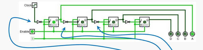
When the clock cycles from high to low (2<sup>nd</sup> cycle):
