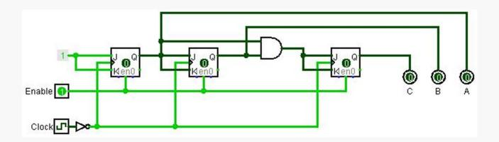
As the clock signal runs, the circuit will cycle its outputs through the values 000, 001, 010, . . . , 111 and then repeat the pattern.
