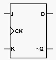
In Logisim and the following diagrams, the JK flip-flops update state on the rising edge (when the clock goes from low to high).
