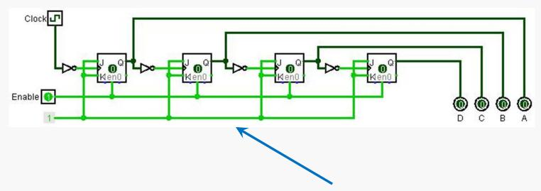
Note that the J and K inputs are all set to the fixed value 1, so the flip-flops "toggle".
