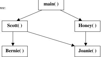
Assume that the software system is to be decomposed for compilation into three separate source files main.cpp, Scott.cpp, and Honey.cpp, and accompanying header files of the same names. The function definitions are to be placed in the various cpp files as shown below along with the corresponding code for the files.
