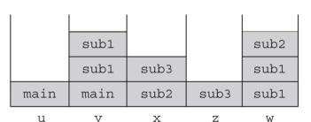
(The names in the stack cells indicate the program units of the variable declaration.)
