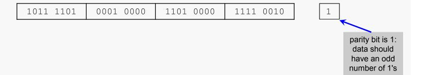
A 1-bit parity code is a *distance-2 code*, in the sense that at least 2 bits must be changed (among the data and parity bits) produce an incorrect but legal pattern. In other words, any two legal patterns are separated by a distance of at least 2.
