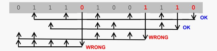
So, what does that tell us, aside from that something is incorrect? Well, if we assume there's no more than one incorrect bit, we can say that because the incorrect parity bits are in positions 4 (0100) and 8 (1000), the incorrect bit must be in position 12 (1100).
