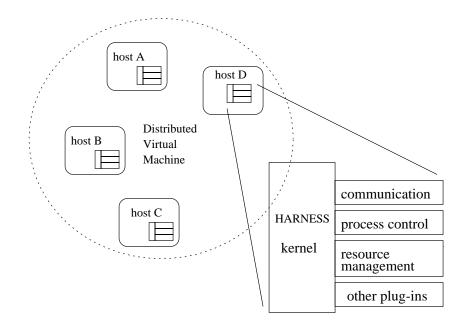
Figure 2: Distributed Virtual Machine is composed of kernels running on each computer and each kernel is composed of 3 required modules (plus possibly others)
