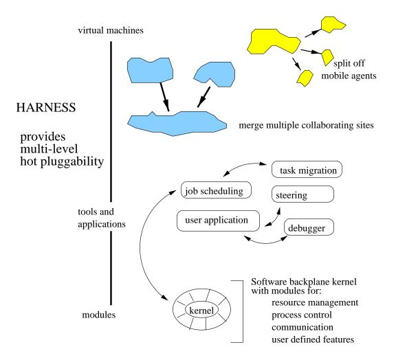
Figure 1: HARNESS allows dynamic plug-ins at module, tool, and virtual machine levels
