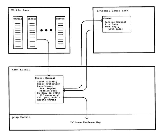
Figure 5-1: Fault Handling
